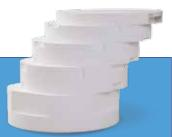
Zirkonzahn-Notch-style BruxZir Milling Blanks are Zirkonzahn Mill 96 mm in diameter at 10-mm thick and keyed for Zirkonzahn milling machines. Thickness size beyond this 10-mm band encircling the blank is machined with three semicircle notches at 120-degree intervals
